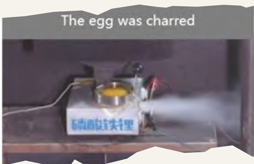
2 BYD Europe’s official website showcases how its Blade Battery has notably passed the “nail penetration test”, one of the most stringent safety tests in the industry.
